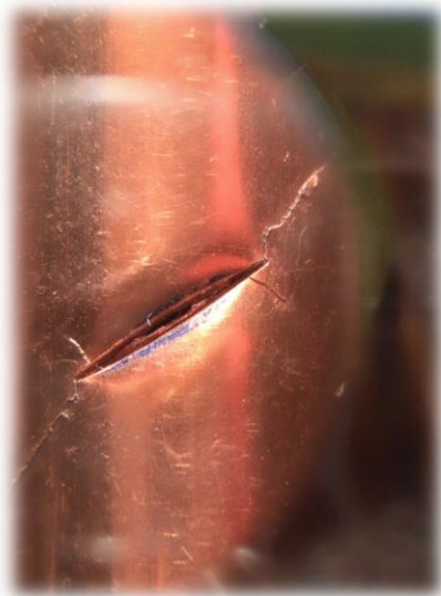
Figure 4. Illustrates a sample of crack path due to torsion cyclic load for the case of \alpha=60 .
