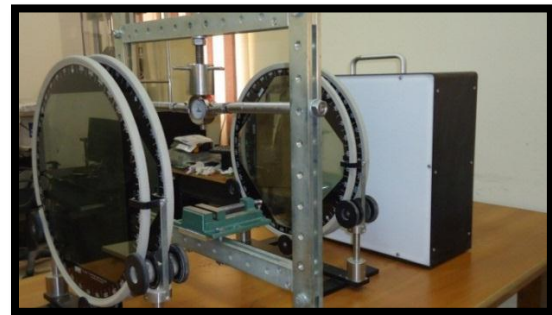
Fig. 4 Transmission circular polariscope and loading frame.
