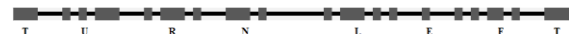
Fig. 3: The pulse pattern of Morse coded alphabet C (figure on top) and Morse coded words TURN LEFT (figure on bottom).
