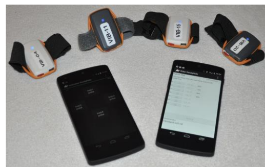
Fig. 2: Ready-Ride: two smart phones (sender and receiver) plus four vibrators in plastic holders.
