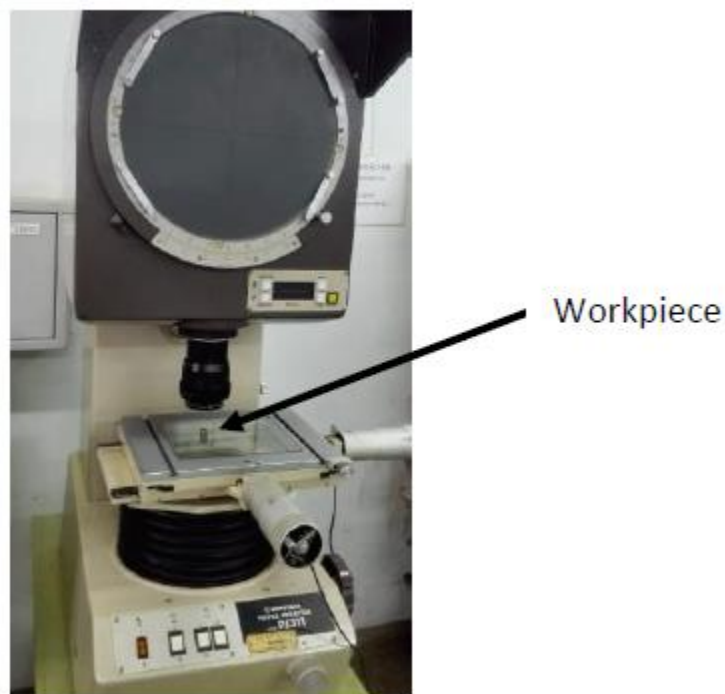
Fig. 4: Setup for measurement of kerf width using profile projector
