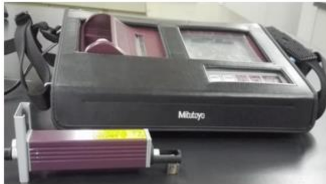
Fig. 3: Setup for measurement of surface roughness using Mitutoyo surface roughness tester
