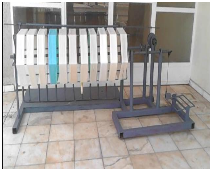
Figure 4: Fabricated manual hank reeling machine (Photo shoot by Author)
