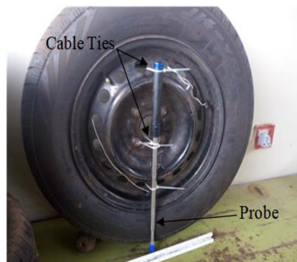
Figure 7: Telescopic probe for measuring deflection at impact
