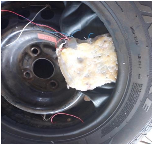
Figure 5: Placement of the patch
